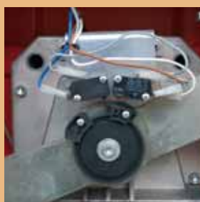
Perfect movements thank to three limit switches
